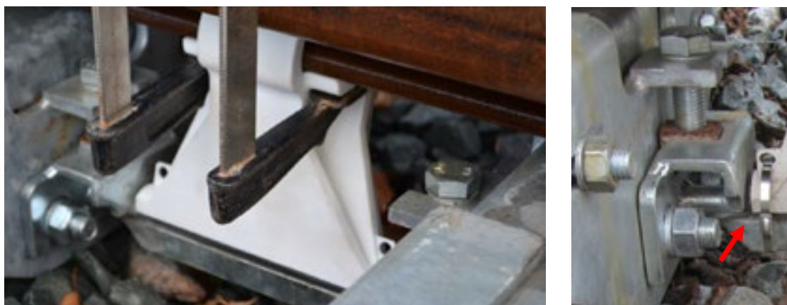
Figure 6a: The pendulum block is clamped against the switch rail using two glue clamps (right: stainless steel tie-wrap)
