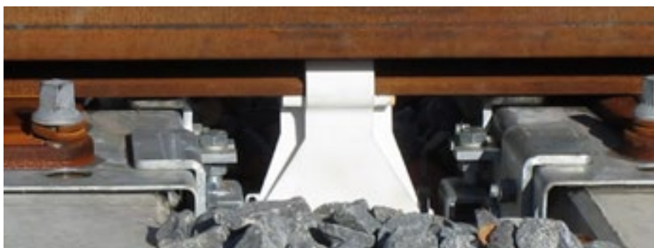
Figure 11: DeltaSwitch pendulum block under the switch rail reinforcement (rectangular tube)
