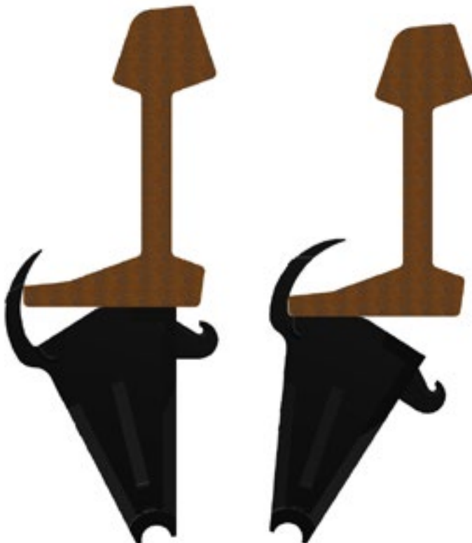
Figure 3: Switch rail resting on the pendulum in both extreme positions.: descending (left) and closed (right)
